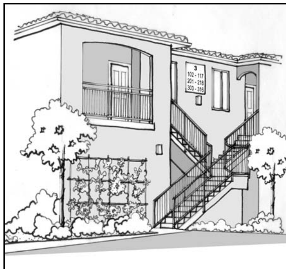
Open stairways allow natural surveillance
