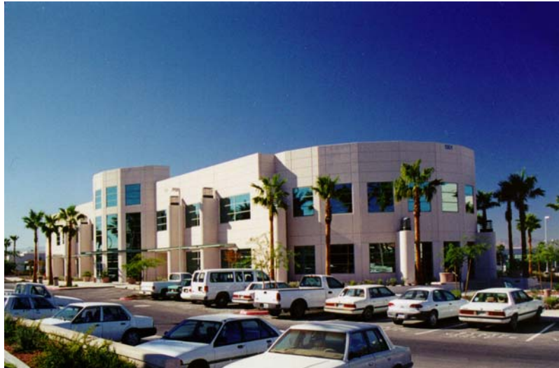
Varying building massing and height, wall offsets, and multiple windows help to reduce the visual mass of buildings.
