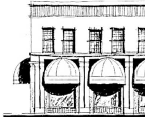
Dome-shaped awnings are not appropriate with rectilinear window openings.
