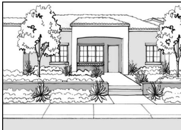
Grade separation and low retaining walls establish a public/private edge and define territories
